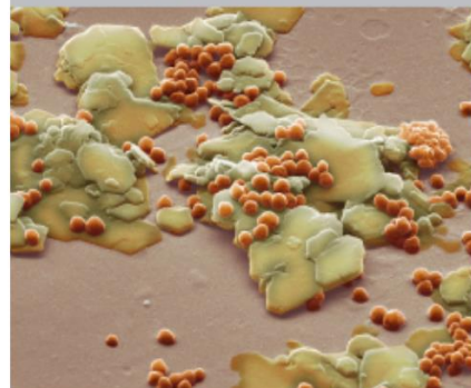
Polyethylene microbeads (orange, shown with yellow flakes of silica) are used as exfoliants in many personal care products. In June 2014 Illinois became the first U.S. state to ban the manufacture and sale of products containing microbeads, which are small enough to slip through filters of wastewater treatment plants. 14 © Steve Delaney/Science Source
